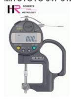
Measurement applications Allows simple, quick and accurate thickness measurement. Features Thumb lever to lift spindle Measuring faces are hardened, ground and lapped Large LCD display Imperial/Metric conversion ABSolute feature Zero/ABS Preset Tolerance setting Counting direction Magnification judgement results
